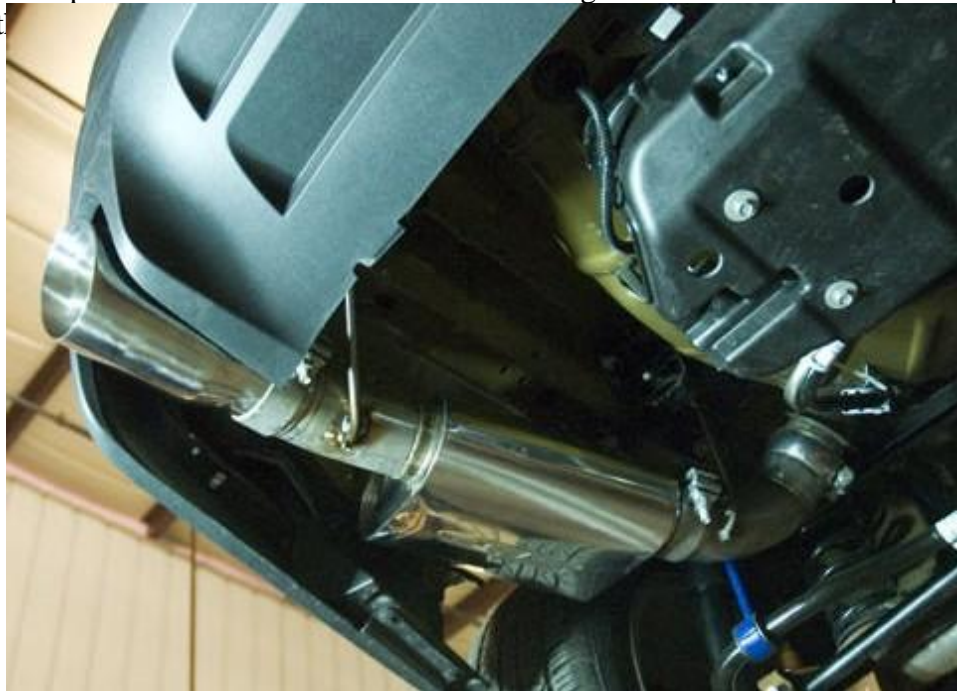
Figure 1: Installation of DS Muffler Assembly
