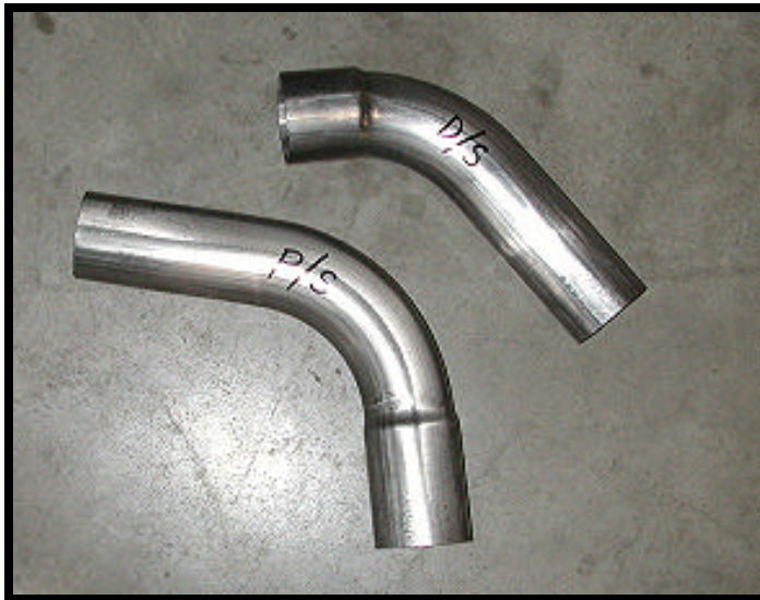
Photo 9: Over-Axle to Tailpipe Connecting Pipes
