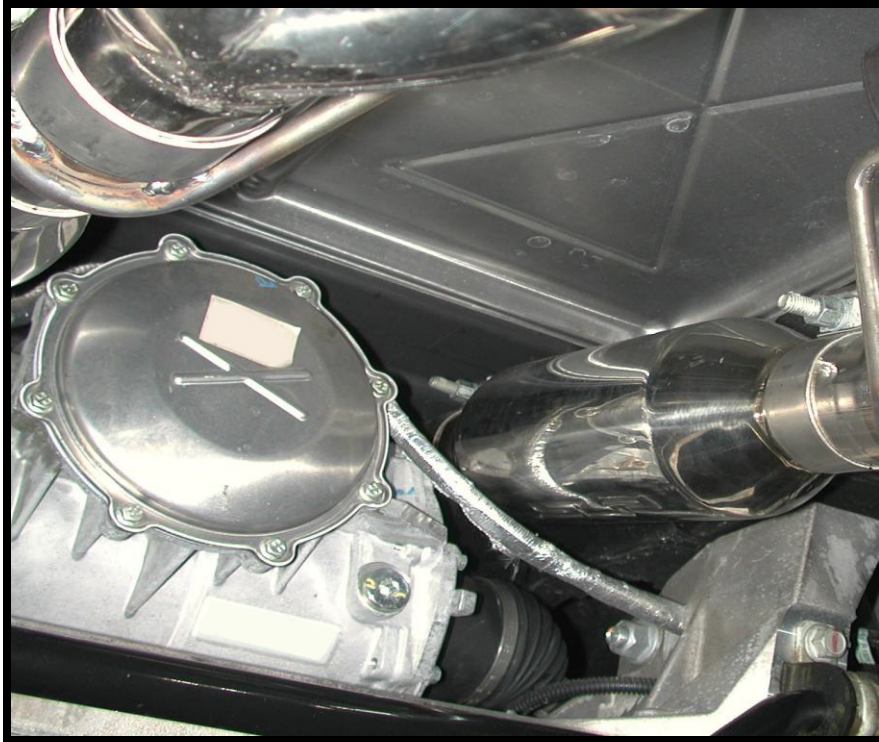
Photo 5: Resonators/Mufflers Installed on Over-axle Pipes
