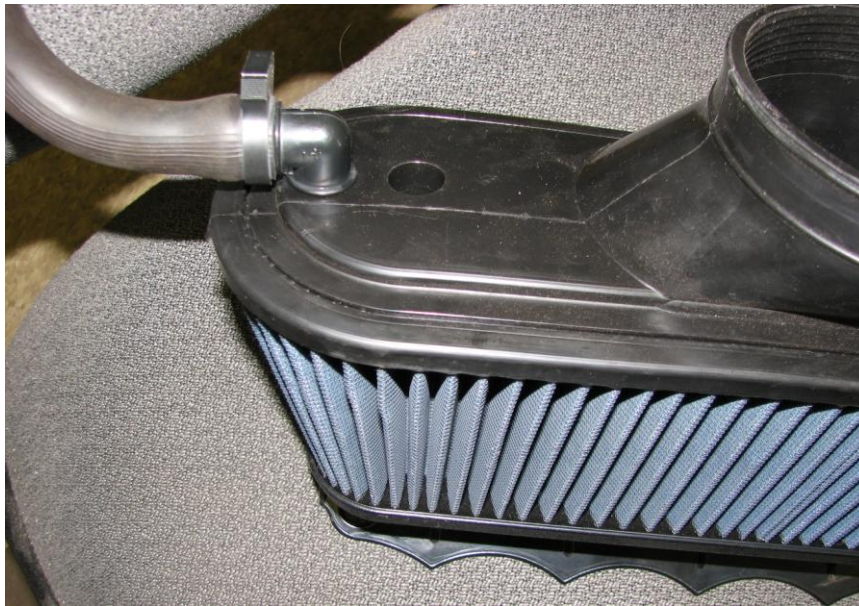
0.75" diameter hole for AIR pump (if equipped)
