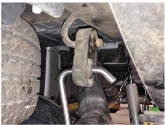
**NOTE:** Remove all of the protective plastic film from the muffler (P/N: 1115-5230) before installing.
