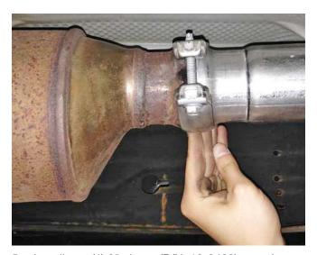
Install one (1) 3" clamp (P/N: 10-0439) over the outlet of the over-axle pipe and install the tip (P/N: 310305787) onto the outlet end of the overaxle pipe. Position and orient the tip to the desired location. Position the clamp on the joint and tighten to 30 Nm.
