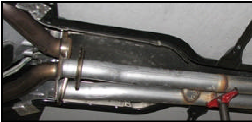
Photo 1: Factory H-Pipe Removal
