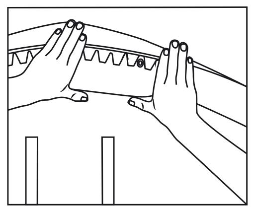
Using your sharp scissors, cut any marked SLIPLO pieces from the previous step. Double check the fitment of each cut piece against the surface. Remember to cut only as much excess material as necessary, ensuring maximum bond integrity of each individual piece.
