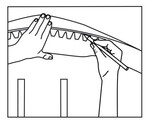
Do not remove any of the red adhesive liner during this testing segment. Place your first piece of SLIPLO up against the surface area you want to protect. Generally, a good rule of thumb is to start from the center of the bumper and test each consecutive piece, moving towards the driver side of the car. Use your pen to mark any overlaps, screws, and holes on the SLIPLO piece which require any type of cutting. Once satisfied, move onto the next piece and repeat.
