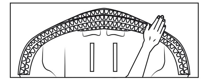
Always take extra care to install the adhesive section of SLIPLO on a flat surface, ensuring that there won't be any pop ups in the future. Install all of the remaining pieces of SLIPLO, ensuring the protection of the front lip impact area of your bumper. Go over and firmly press each piece down using the palm of your hand insuring that adhesive is fully activated.
