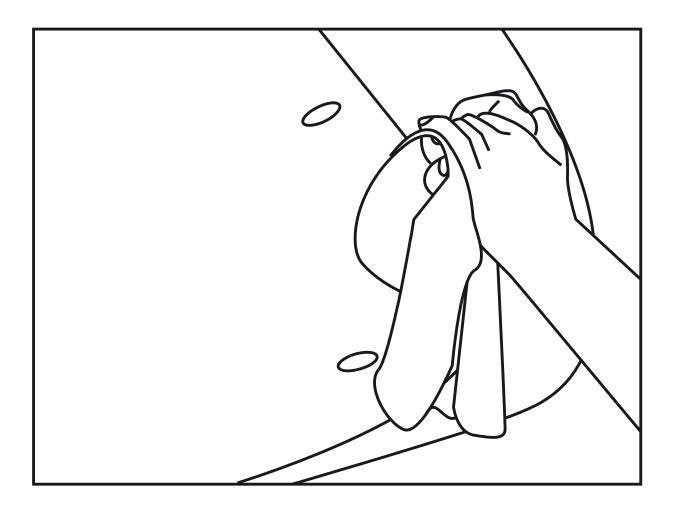
Use the 70% Isopropyl alcohol (IPA) and a towel to clean the surface of any oily layer or contamination on your car. Where heavy oil, grease or a ceramic coating is present, a "degreasing" solvent such as gasoline can be used to remove any contaminants. However, take extreme care not to damage the paint.
