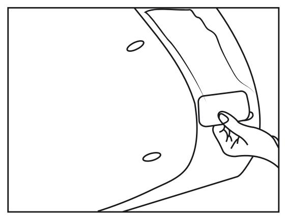
Make sure to use a glove when handling any type of adhesive promoter. Quickly apply a single thin layer of the adhesive promoter to the surface area using the applicator sponge. Make sure to let the surface sit until fully dry before moving onto the next step. If the surface has pre-existing damage, make sure you focus on these areas with the application of extra promoter.
