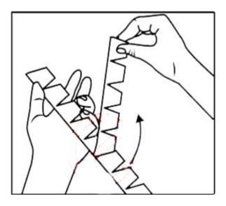
Remove the adhesive red liner from the back of the SLIPLO piece.
