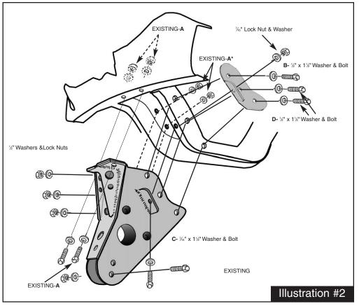
remove the original radius arm frame brackets and remove from front axle housings.
