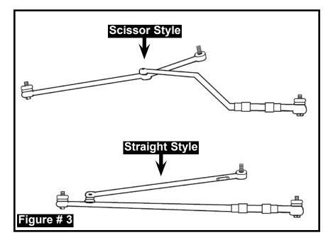
76-77 Ford F100 / F150 & Bronco. The drag link & tie rod assembly will require changing to the "Straight Style" steering in order to install a drop pitman arm. (See Figure # 3)
