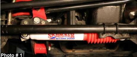
6. After installation be sure to cycle the steering & check for adequate clearance. In most cases the OEM steering stabilizer bracket on the tie rod assembly will need to be rolled down slightly to allow for adequate clearance.
