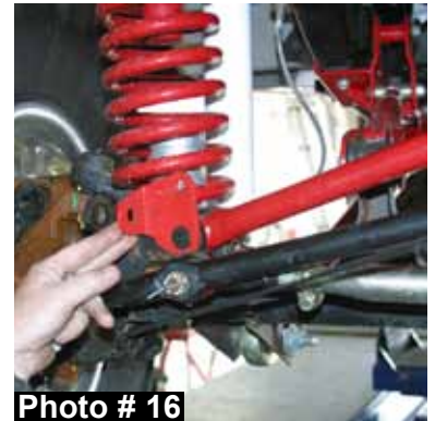
5/16" x 3/4" thread cutter flange bolt.
