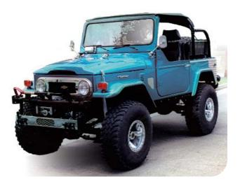
Make sure you park the vehicle on a level concrete or asphalt surface. Many times a vehicle is un level (side-to-side) from the factory, but usually not noticed until a lift kit has been installed which makes the difference more visible. Using a measuring tape, measure the front and rear (both sides) from the ground up to the center of the fender opening above the axle. Record below for future reference.
