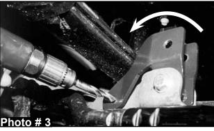
Here's A Tip: Have a friend turn the steering wheel slightly from left to right, this will aid in aligning the trackbar to the trackbar bracket hole. See arrow below.
