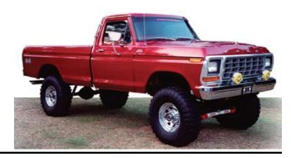
Make sure you park the vehicle on a level concrete or asphalt surface. Many times a vehicle is not level (side-to-side) from the factory & is usually not noticed until a lift kit has been installed, which makes the difference more visible. Using a measuring tape, measure the front & rear (both sides) from the ground up to the center of the fender opening above the axle. Record this information below for future reference.
