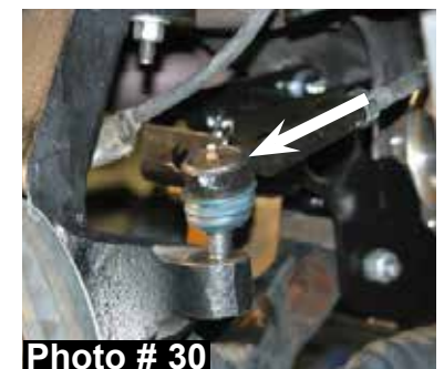
Passenger side shown with one 15/16" cv-spacer.
