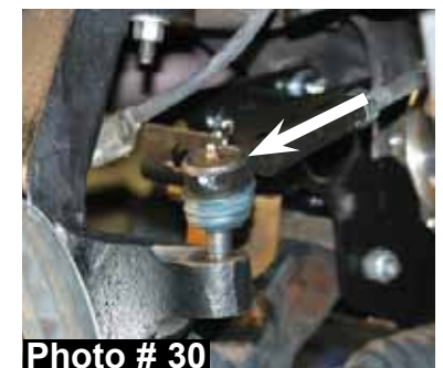
Passenger side shown with one 15/16" cv-spacer.
