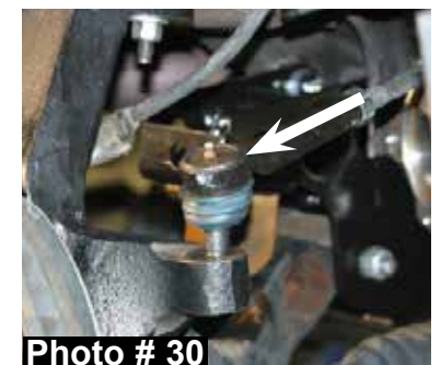
Passenger side shown with one 15/16" cv-spacer.
