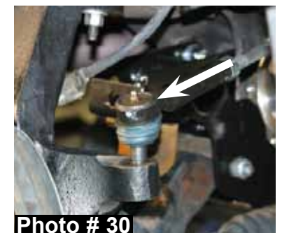
Passenger side shown with one 15/16" cv-spacer.
