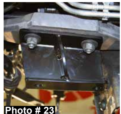
Photo # 23 Arrow shows the support shim from Step # 24. Found in hardware bag Part # HB-C9682FDB
