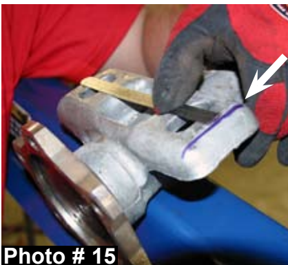
REAR mounting point on passenger side diff tube.
