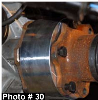
Driver side shown with 3.35" cv-shaft spacer.
