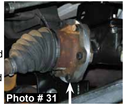
Photo # 31 Passenger side shown with one 15/16" cv-spacer.
