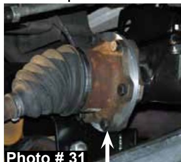
Passenger side shown with one 15/16" cv-spacer.
