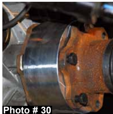
Driver side shown with 3.35" cv-shaft spacer.
