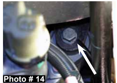
Photo # 14 REAR mounting point on passenger side diff tube.
