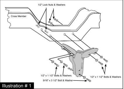
7. Install the supplied 1/2" x 1 1/2" bolts, washers, & nuts labeled as "B", through the new Skyjacker bracket & cross member. Pivot the bracket down so the tab is flush against the cross member lip. Drill a 7/16" hole, for bolt labeled as "C" & install the supplied 7/16"x 1 1/2" bolt, washers, & nut
