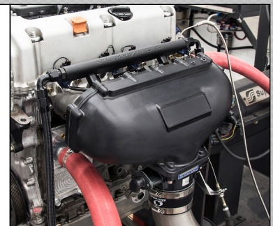
Skunk2 engineers produce a series of virtual 3D manifold models, and then use Computational Fluid Dynamics (CFD) to simulate and analyze the behavior of airflow. Prototype manifolds are tested on engine dyno until the design is optimized.
