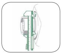
Clean and measure the diameter of the worn shaft and mark the area where the sleeve will cover the scored portion of the shaft.
