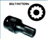
This special socket was designed for R&R of Tamper-Proof type transmission drain plugs. The 16mm "XZN" pattern socket has a security hole in it and a 1/2" drive. Made from solid steel.
