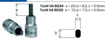
These special "Oval-Pin" drive Bits with a 1/2" drive, were developed for the crucial task of prying open the strut clamps of hub castings in order to free the bottom of the strut unit.
