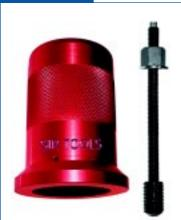
This Special Kit was designed for the proper installation of **Pulley Crank Shaft** oil seals. The step bolt screws into the crank shaft end. The press nut w/ washer allows for an even pressing force, seating the oil seal into the engine case every time. **Applicable:** Most Honda / Acura
