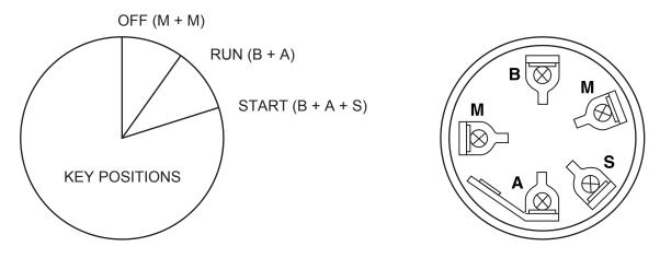
A-ACCESSORY B-BATTERY C-CHOKE (Electric)
