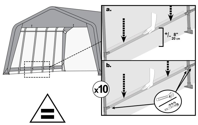
Simultaneously tighten ratchets 1 & 2, then 3 & 4.
