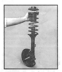
10. Reassemble all components in reverse order. Be sure Coil Spring Seats are reassembled so that they match ends of Coil Spring. Loosen each leg evenly and allow the ends of Coil Spring to contact the seat properly. Remove each leg. Repaired MacPherson Strut is now ready to be reinstalled on vehicle.
