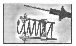
**9.** Remove coil spring in compressed condition and set aside. Shock Absorber is now exposed to be fixed or replaced.
