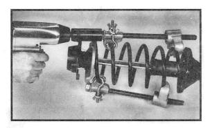
7. Compress coil spring using hand tool or impact gun with 15/16" socket. Turn each bolt alternately so that compression of spring is equal on each side. Compress until the ends of the spring are completely free of the spring seats at each end of the coil. Total compression required is usually not more than 3".
