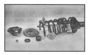
8. Remove Upper Bearing Dust Cap on MacPherson Strut to expose Piston Rod Nut. Remove Piston Rod Nut, Upper Bearing Plate and Upper Coil Spring Seat.
