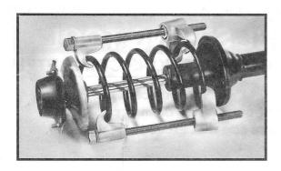
**5.** Affix second leg of tool on opposite side of coil spring in same manner as done for first leg. Hand tighten bolt.
