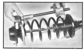
**3.** Affix one leg of tool as shown. Hooks on both ends of leg should engage coil spring so that furthest rungs are held by hooks.
