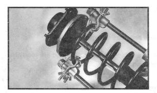
6. Apply Safety Hooks to spring with flange and wing nuts. Assemble to each leg and coil spring as shown. Wing Nuts should be finger tight.
