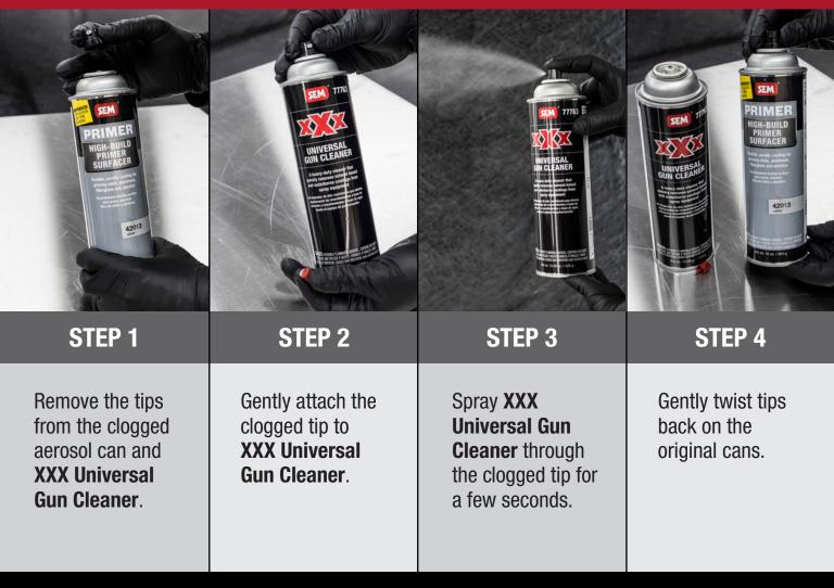
NOTE: This technique can be used with any aerosol product that is prone to clogging. 77763 XXX Universal Gun Cleaner will not damage plastic comfort tips.
