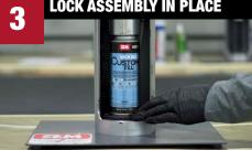
Place assembly into machine. Hold cylinder and can assembly in place and tighten pedestal on bottom. Close door on Custom Fill Machine.
