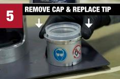
Remove cylinder/cap assembly from machine. Twist gently to remove cylinder from can. Hold cylinder and press down on a hard surface to remove cap. Replace tip.
