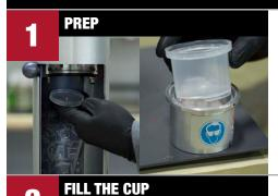
Remove disc from cap and insert over piston inside the fill machine. Place clear plastic cap into the Fill **Cylinder.** Press down and rotate cap until it drops into place.
