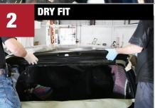
Dry fit all panels to ensure proper alignment. Drill holes for replacement rivets or mark locations of self-piercing
