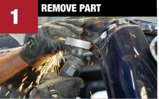
Remove spot welds with spot weld cutter. Remove rivets by drilling or grinding. Remove damaged panel and straighten bent flanges with a hammer and dolly.
