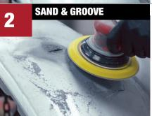
On front side, sand repair area with P80 grit. Dish out damage with P36 grit disc at a low RPM. On back side, grind repair area with P36 grit disc at a low RPM. Blow off surfaces. Re-clean if necessary.
