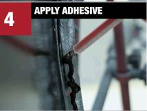
Apply 3/8" - 1/2" bead of **Dual-Mix**<sup>TM</sup> Multi-Purpose Panel Adhesive or **Dual-Mix Weld-Bond Adhesive** to both surfaces. Use enough material to completely fill the joint when parts are clamped. Tool with a spreader or acid brush. Cover all exposed bare metal.
