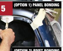
Clamp panel into place. Do not over clamp. Wipe away excess material.
