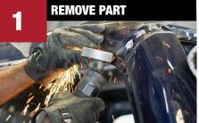
Remove spot welds with spot weld cutter. Remove rivets by drilling or grinding. Remove damaged panel and straighten bent flanges with a hammer and dolly.
