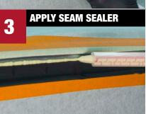
Apply **SEM 2K Seam Sealer**. Immediately smooth or tool **Seam Sealer** to match OEM texture.
