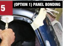
Clamp panel into place. Do not over clamp. Wipe away excess material.
