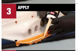
Apply **1K Seam Sealer** using **1K Pneumatic Applicator** or a manual applicator. Finish with a gloved finger, acid brush, putty knife, or spreader.
