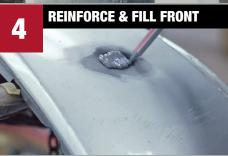
Remove tape from front. Fill front with **Dual-Mix Multi-Plastic Repair Material** or **Dual-Mix Problem Plastic Repair Material**. Spread material firmly and build up higher than panel to allow for sanding. Allow to set before sanding.
