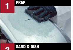
Clean front and back with **Scuff & Clean** and damp, gray scuff pad. Rinse with water and dry or wipe with a clean, damp cloth until removed. Clean front and back with **SEM Solve, Plastic & Leather Prep** or **XXX Universal Surface Cleaner**. Wipe clean in one direction with dry, lint-free cloth.
