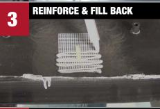
Mask front side of repair to prevent repair material from flowing through. Apply **Plastic Repair Contouring Tape** (mesh only) to back side. Apply **Dual-Mix™ Multi-Plastic Repair Material** or **Dual-Mix Problem Plastic Repair Material** and cover mesh tape. Spread material firmly. Allow to set.
