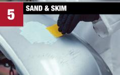
Sand with P80 grit. Finish with P180 grit. If needed, use a skim coat of **Bumper Bite™ Flexible Glaze**, then sand with P180 − P320 grit.
