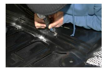
**Step 8:** Carefully tip or raise the carbon hood to find the fiberglass piece that should have fallen after the indentation was punctured.
