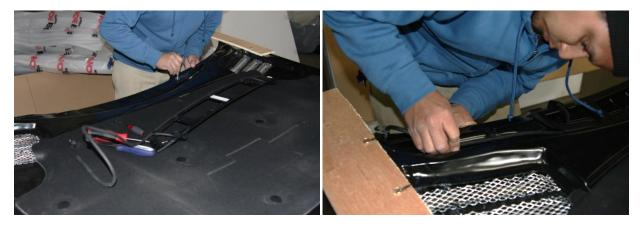
**Step 12:** In some cases, depending on the vehicle you have, you may have to/want to transfer your OEM striker onto your new carbon fiber hood. To do this, simply unbolt the striker and screw it onto the carbon hood.
