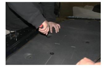
**Step 6:** Place the heat shield over your carbon hood- this will give you an idea if minor adjustments may be necessary. In this case we used a dremel to cut along the sides of the indentations that were on the carbon hood. Be careful when cutting so you do not cut through the hood.
