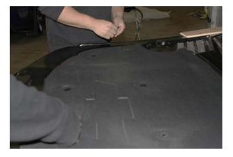
**Step 10:** If you want to install windshield washer nozzle, carefully remove the windshield washer hose from the OEM hood by unclipping it. You may have to twist and wiggle it around. Be sure to also remove the plastic frame that is attached to the hose (if applicable).
