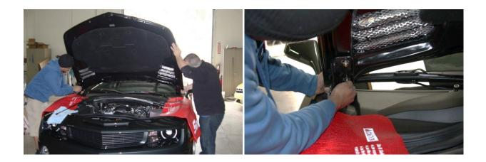
**Step 13:** Before closing the hood, make sure the fenders are clear and that there are no tools left in the engine bay. Carefully close the hood. Slamming the hood may cause it to crack. Check alignment of the hood and latch. If satisfactory, the hood installation is complete.
