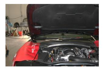
**Step 2:** Remove the OEM factory hood by removing the bolts/nuts attaching it to the hinge. (Note: You may have to remove any garnishes that are part of the OEM hood). You will need help from a partner to hold the hood while you are unbolting it.
