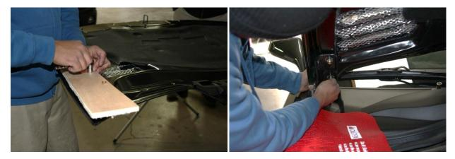
**Step 4:** Look at the underside of the hood. At this point you want to determine whether you can transfer your OEM heat shield onto your carbon fiber hood. The hood's style will determine if a heat shield transfer is possible. **If you cannot transfer the heat shield, proceed to step 10.** Be advised that you can purchase an aftermarket heat shield online. The use of a heat shield will help protect your carbon hood from damaged caused by engine heat.
