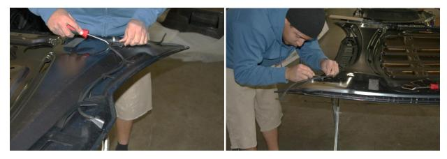
**Step 11:** Transfer the windshield hose and its frame over to the carbon hood. It may be necessary to enlarge the mounting points - you can do this by using a small file.
