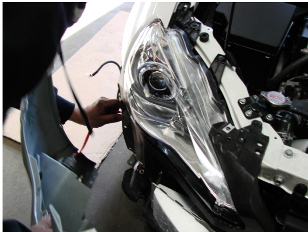
Remove the connector on the vehicle side
