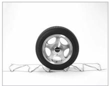
Move the chain in a sweeping motion under the vehicle so the open mid-section is positioned against the backside of the tire. This sweeping motion can best be done while kneeling in front of the tire.
