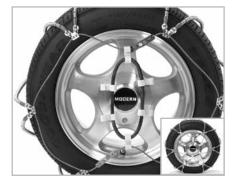
Attach the rubber tensioner to take up the additional slack. To make this simpler, attach the first hook at the "6 o'clock" position, the next at the "12 o'clock" position and so forth. The open side of the hooks must face away from the tire. No further adjustment is necessary.
