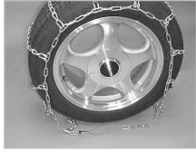
Drape the chain over the tire, again making sure cross chain hooks are facing upward. Hooks that face down (towards the tire) will cause damage to the tire.
