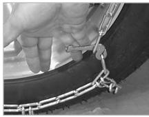
Next fasten the outside fastener, making sure it is as tight as possible. Drive a short distance and retighten all fasteners. For best results, make sure fasteners are adjusted equally and as tight as possible.
