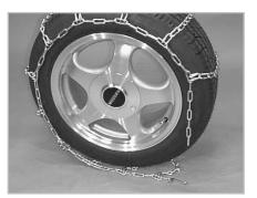
Drive forward a few feet, far enough so that one or two of the cross chains pass under the tire.
