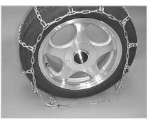
drape the chain over the tire, so that one cross chain is positioned at the point where the tire meets the ground. Again make sure the cross chain hooks are facing upward. Hooks that face down (towards the tire) will cause damage to the tire.
