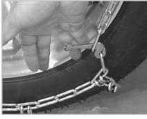
5 Next fasten the outside fastener, again making sure it is as tight as possible. Drive a short distance and retighten all fasteners. For best results, make sure fasteners are adjusted equally and as tight as possible.
