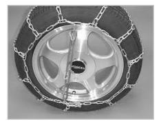
6 SCC recommends chain tighteners (sometimes known as chain spreaders) be used to take up additional slack. To make this simpilar, attach the first hook at the "11 o'clock position", next at the "5 o'clock position" and so forth. The open side of the hooks must face away from the tire. No further adjustment is necessary.
