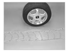
Park vehicle on firm level ground and turn off the engine. Set the parking brake. Unroll the chains and lay them out flat on the ground, making sure there are no twists or tangles. Make sure the cross chain hooks are facing upward.
