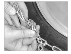
Reach behind the tire and engage the inside connector on the 2nd or 3rd link. See the illustration below for a detailed look at making this connection.
