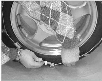
**4** On the outside of the tire, thread the cable with bushings through the end hook for initial mounting. Grasp the outside side cable with both hands and pull it towards you. This will create as much slack as possible. Then make the outside connection in the same manner.
