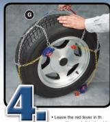
up position and slide the side cable to the back of the tire (G), ensure the chain is centered on the tire.
