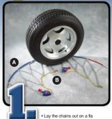
surface, remove all tangles and ensure the side wire hooks are facing down
