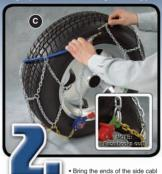
in front of the outer side wall. . Connect the side cable together by inserting the kno into the key-hole latch (C) . Leave the connected side
