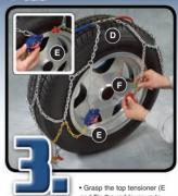
and flip the red lever up to install. Pull the red cable end out and attach to the
