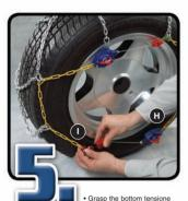
(H) and flip the red lever up install. Pull the red cable end out and connect to the side chain connector (I). PINCH WARNING: Keep your fingers clear of the chain and tensioner while engaging
