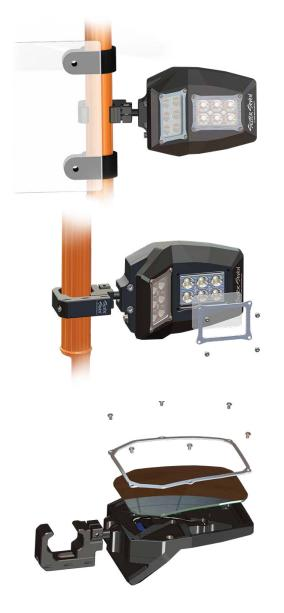
**Do you have a windshield?** | No problem! If installing our Spectrum lights/mirrors on a vehicle with a windshield, simply rotate clamp 180° and install on backside of cage. All other steps are the same.
