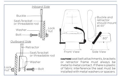
**WARNING:** metal to metal contact is critical on attachment to vehicle structure at brackets and retractor mounting locations
