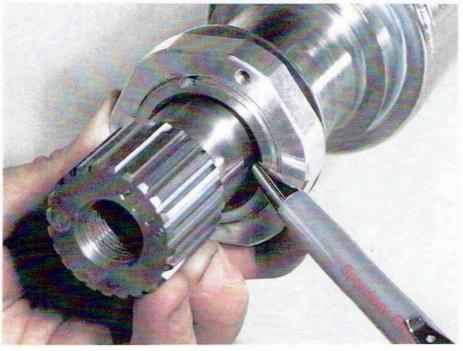
2. The proper axle, with an OD of 1.250° fits easily into the Mod Lite snout, which has a 1.375° ID. Carefully push it in and check the clearance between it and the snout. The  $\frac{1}{4}$ ° (0.125°) clearance should be visible to the eye and can be felt when you move the axle.
