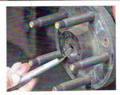
6. Make sure you have an adjustment bolt on the inside end of either the left or right axle when a cross pin isn't used. Without an adjustment bolt, the splines may rub the end of the snout and get damaged. With an adjustment bolt, the axle fits the drive plate and does not move back and forth excessively.  $\overrightarrow{Y}$
