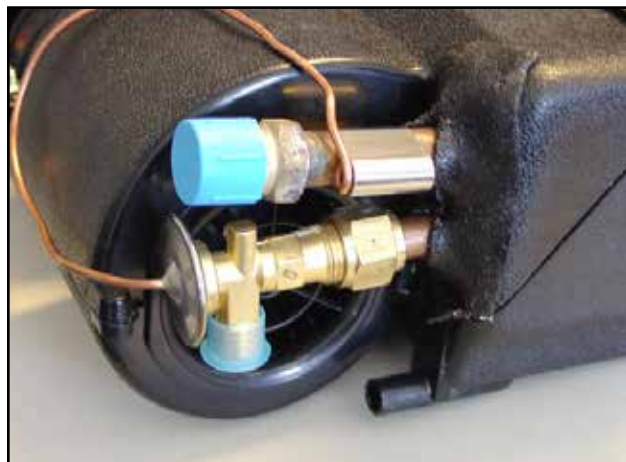
Photo 1 - Install Expansion Valve
