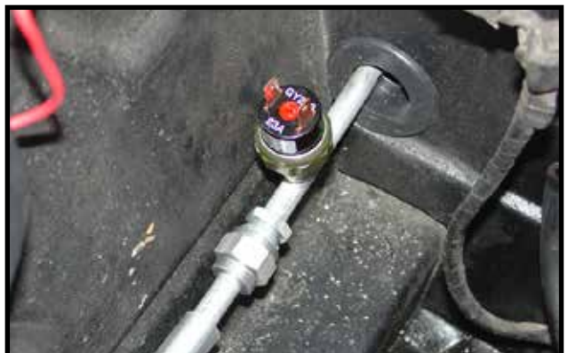
Photo A4 - Pressure Safety Switch
