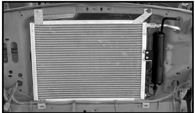
Photo B2 - Mount Condenser Assembly
