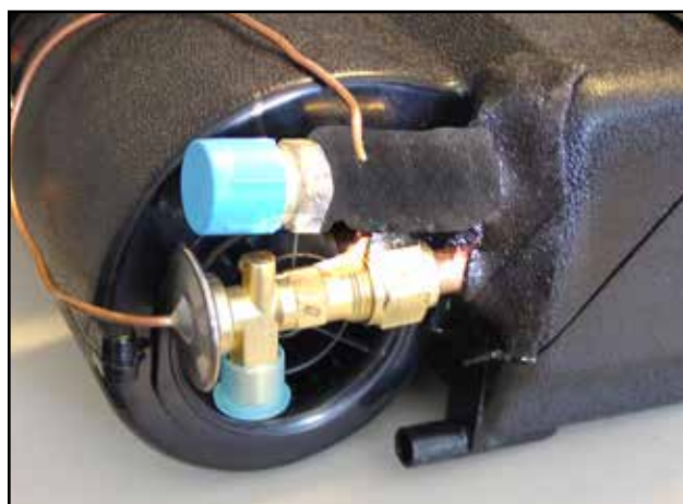
Photo 2 - Wrap Sensor With Insulating Tape
